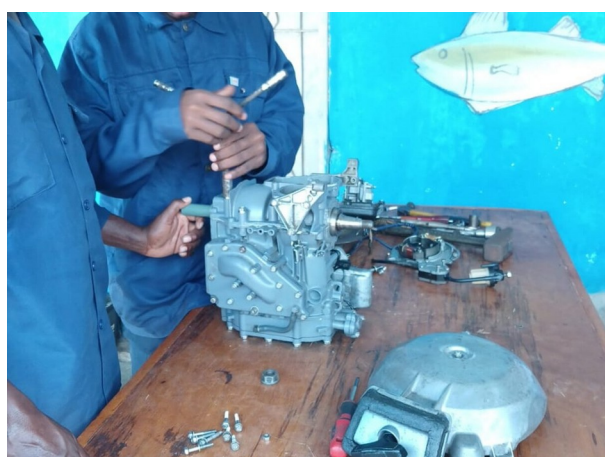
Outboard engine strip-down and repair training in the Institute's workshop.
